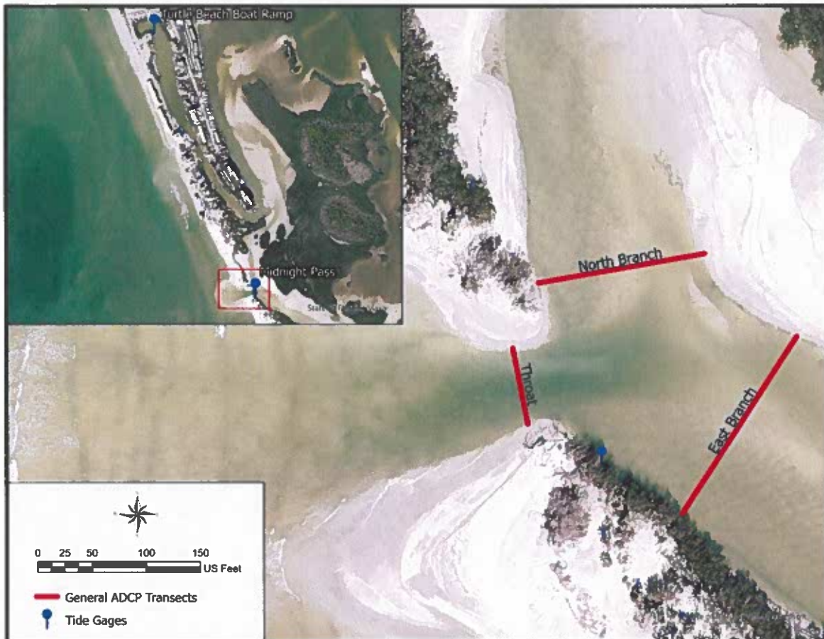
Figure 2. Locations of Pressure Sensors (i.e., Tide Gages) and ADCP Transects where Water Level Data and Flow Data Were Collected, Respectively.
